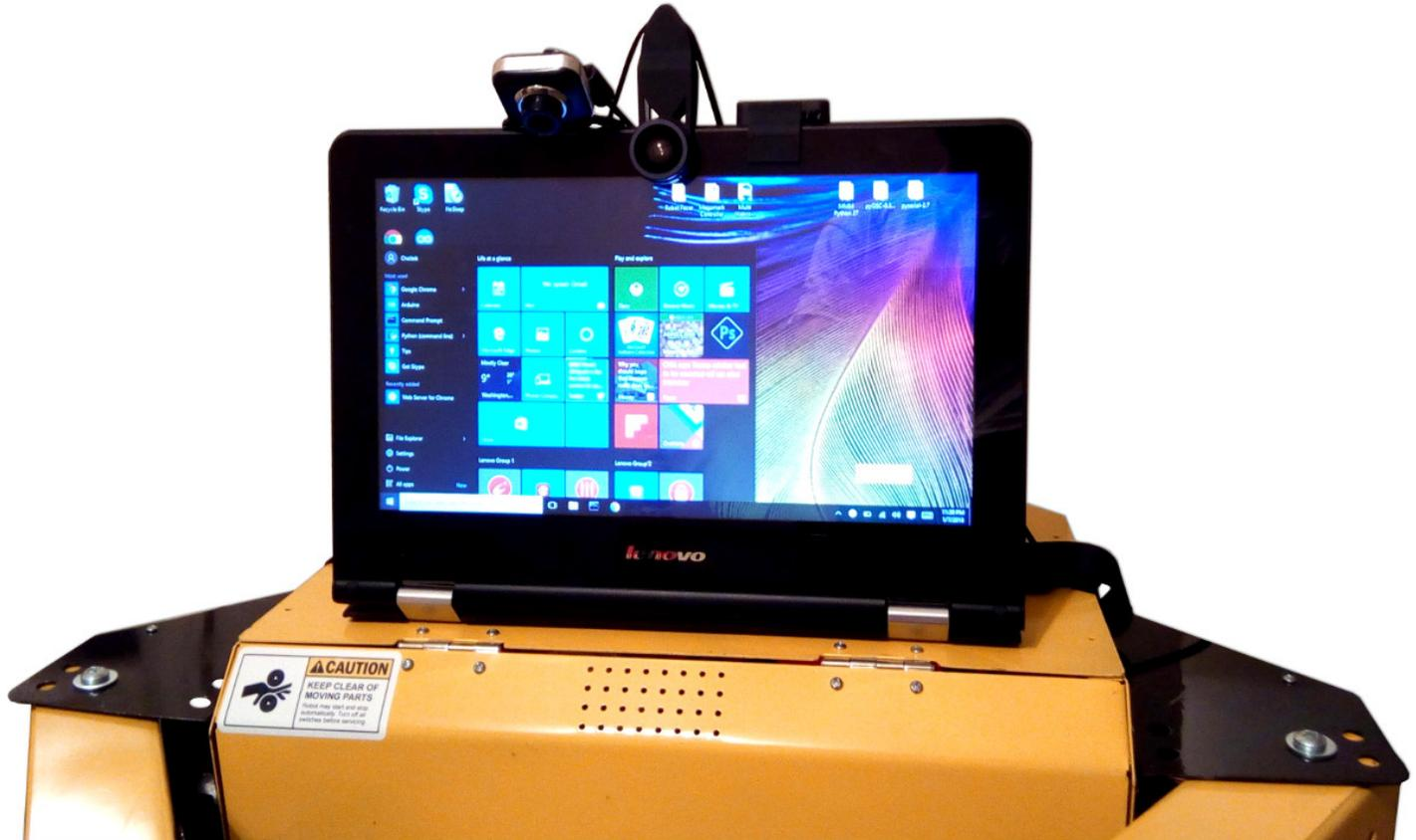
The Choitek Megamark is a hyper-reconfigurable telepresence robot designed to eliminate the high costs of transportation and revolutionize communication by enabling remote collaboration in the office from anywhere in the world, at any time. This guide is designed to show you how you can setup your Megamark robot as versatile, low-cost mobile telepresence solution using a laptop-for-face and free software.
