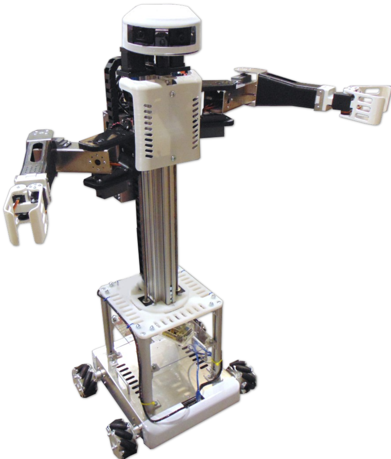
Perspective view of Custom 2-armed Mobile Manipulator Robot Platform
